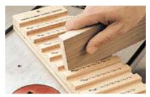
The problem is it takes awhile to find the exact combination of chippers needed to produce a good fit. So I use this handy gauge to tell me at a glance, which chippers to use, see drawing. The gauge is nothing more than two glued-up pieces of 3/4"-thick plywood with a series of dadoes cut in it - one for each different width of dado that I can cut with my blade. The combination of chippers required to cut each dado are labelled underneath.
